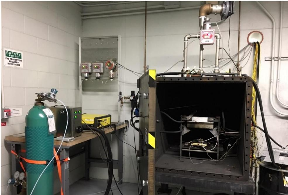
**Figure 13-4 Large Destructive Test Chamber Setup**
