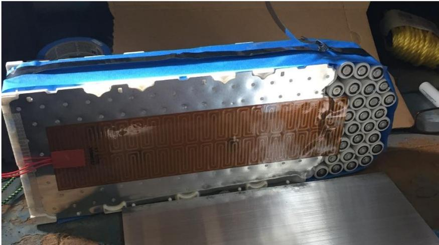
**Figure 14-4 – How (LFP cylindrical) cells were packaged for testing.**
