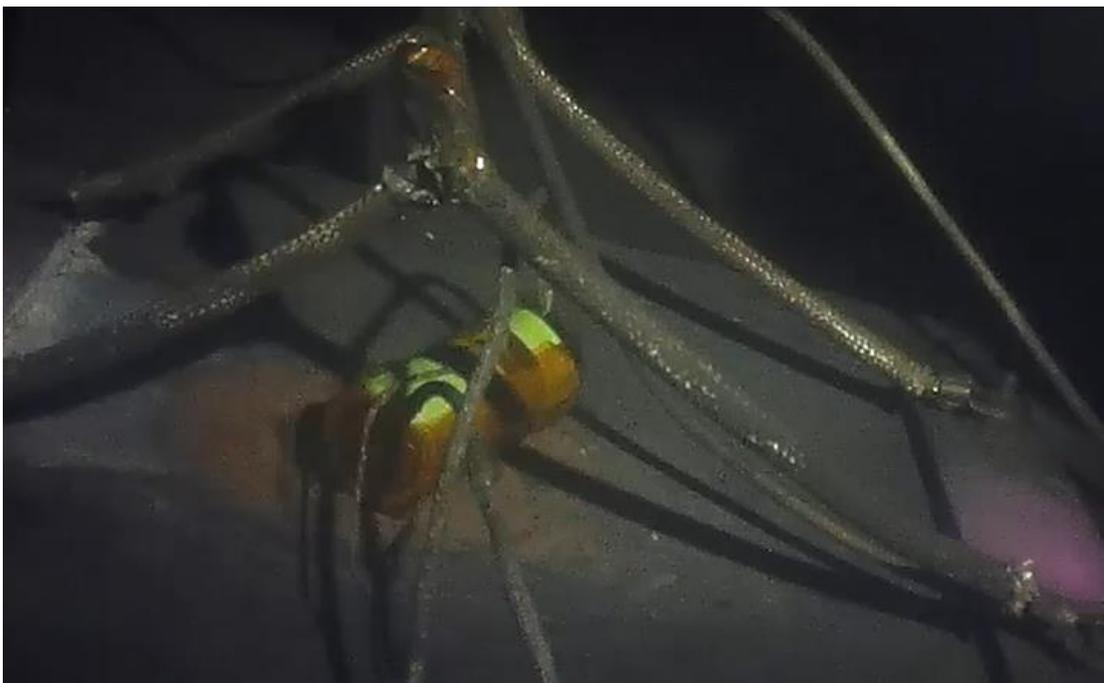
**Figure 13-2: LFP 2.5 Ah cylindrical cell heated up**
