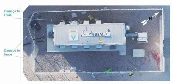
Figure 5 Aerial view of damaged BESS (image credit: Colwell Consulting)
